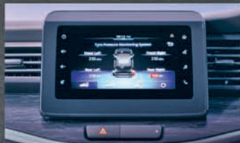
TYRE PRESSURE MONITORING SYSTEM
